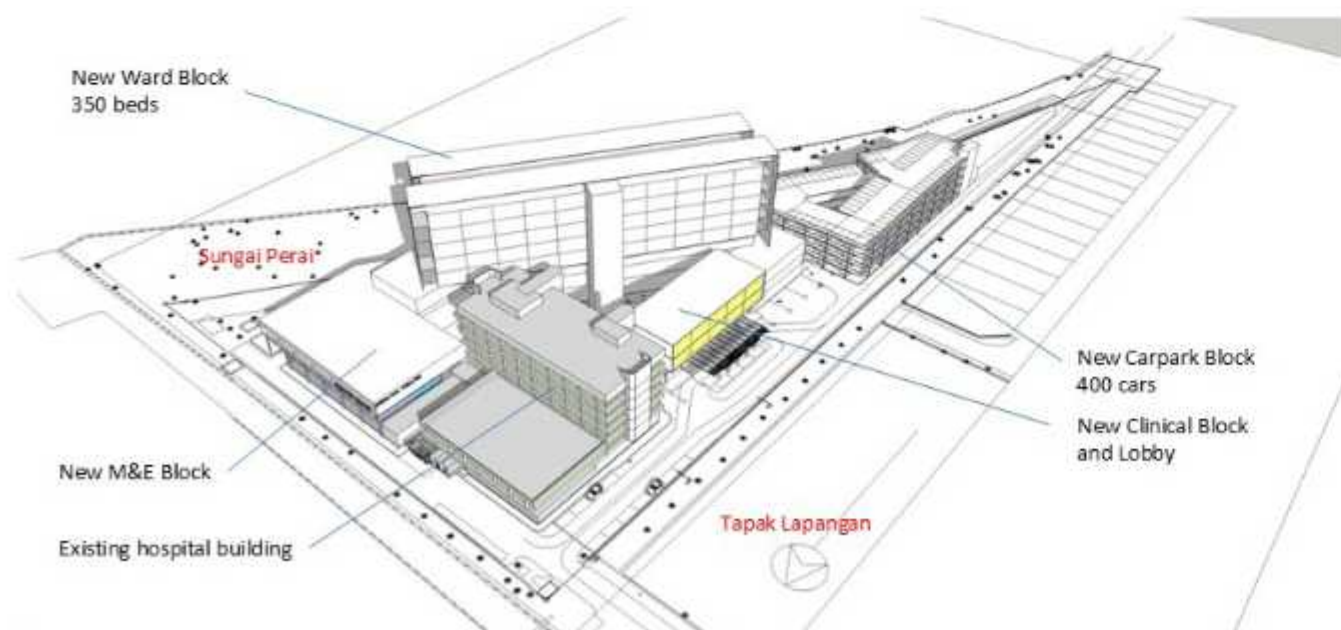
Axonometric view of the hospital complex, used to manage construction sequence, demarcation of departments and traffic flow
