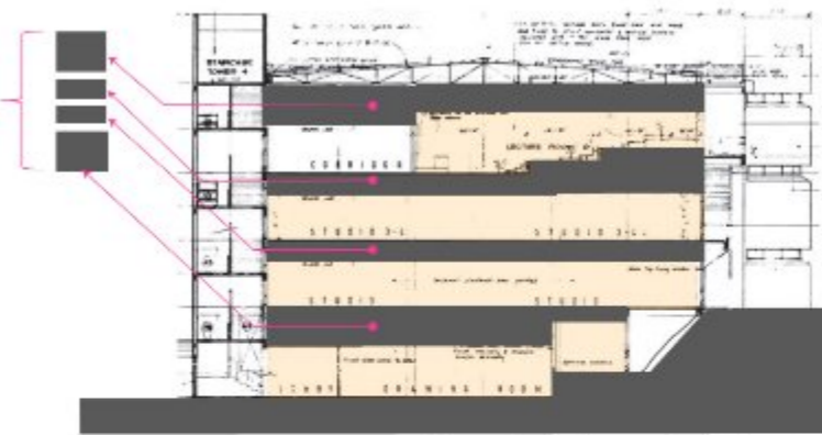
Recovery of volume from removing the false ceiling
